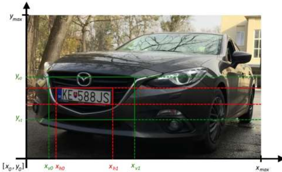
Figure 7 Area detected by vertical projection (green) and horizontal projection (red)
