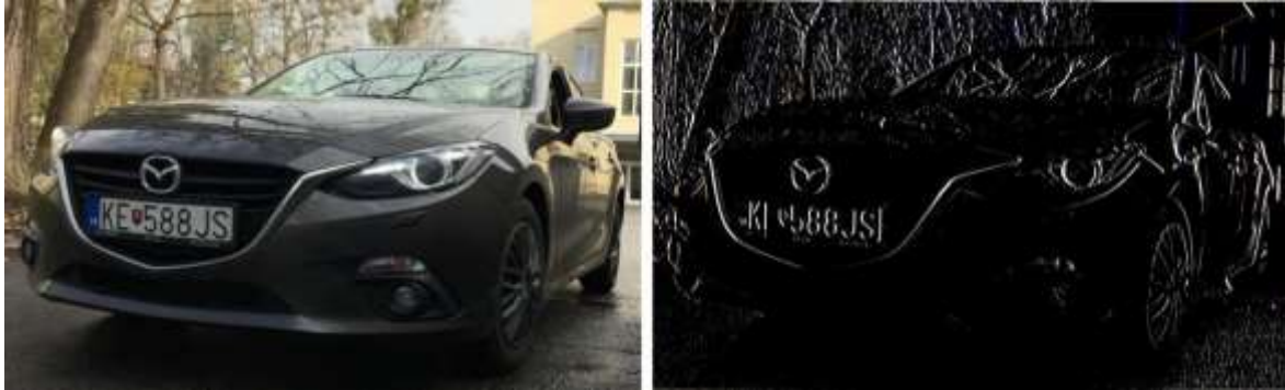
Figure 3 Input frame before and after thresholding
